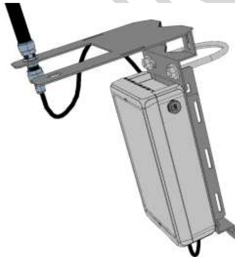
Figure 15 : Another view of the pole mounting using U-bolt (no pole represented)
