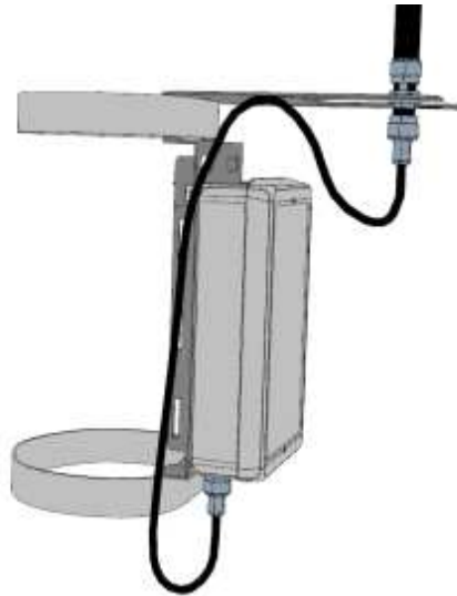
Figure 18 : Another view of the pole mounting using strapping (no pole represented)
