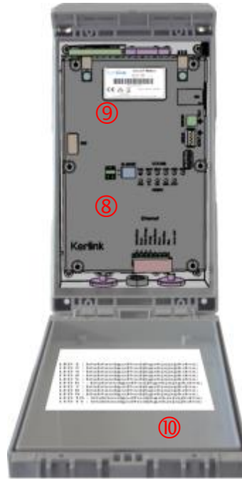
Figure 5 : LoRa IoT Station casing - internal view (temporary image)
