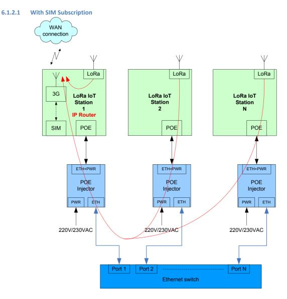
Figure 9 : Multi-station installation (with SIM)
