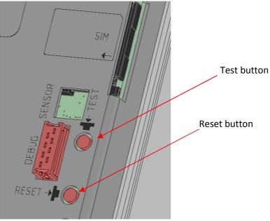
Figure 26 : Test and Reset buttons
