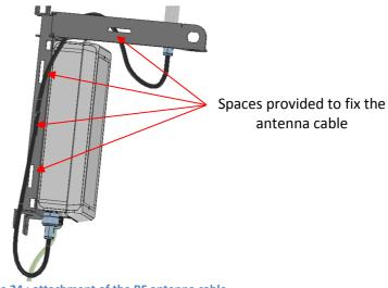
Figure 24 : attachment of the RF antenna cable
