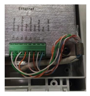
Figure 11 : Ethernet connection
