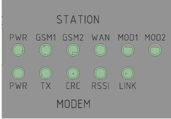
Figure 27 : LEDs indicators
