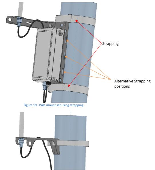
Figure 20 : Pole mounting of the universal antenna support using strapping
