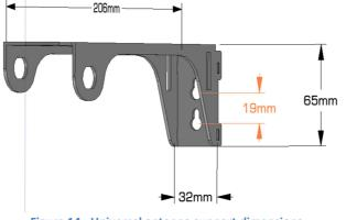
Figure 14 : Universal antenna support dimensions
