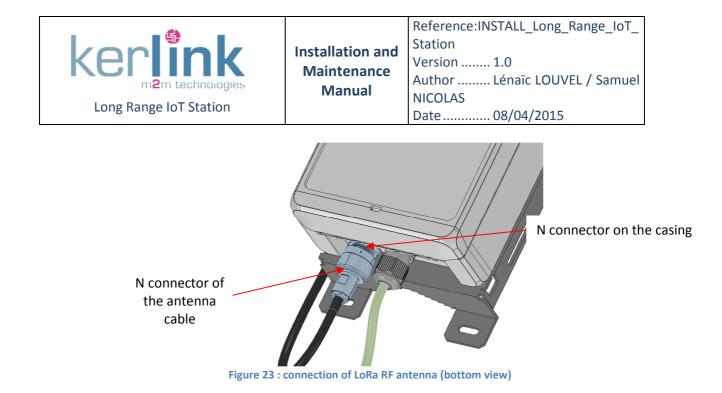
To improve the durability of the RF connections against environmental aggression (moisture, pollution, ...), Kerlink recommends to recover connectors with an insulating tape like the reference 130C from 3M.
