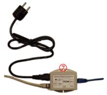
Figure 4 : POE injector (example)
