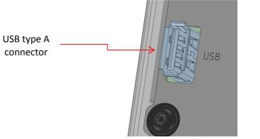
Figure 29 : USB connector of the LoRa IoT Station
