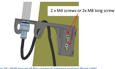
Figure 18 : Wall mount of the universal antenna support (front side)
