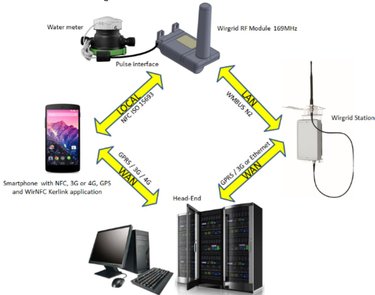
Figure 2: Wirgrid RF Module 169MHz interfaces in the AMR chain
