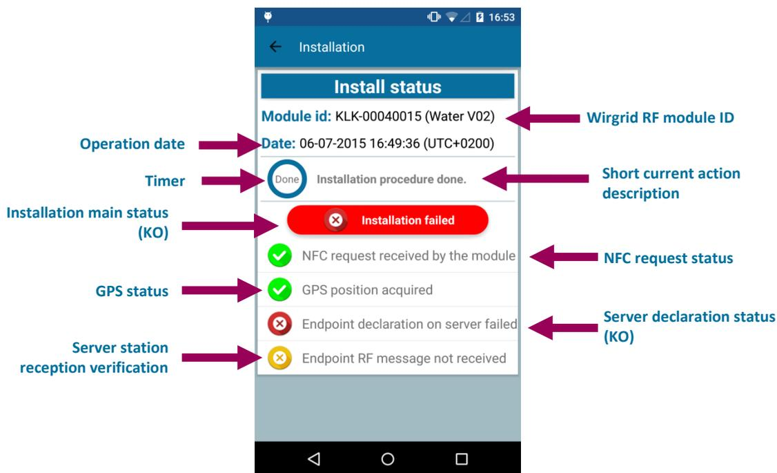
Figure 13: Installation failure (Server declaration failure)
