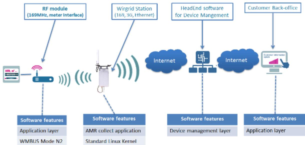
Figure 1: Wirgrid RF Module 169MHz in the AMR chain
