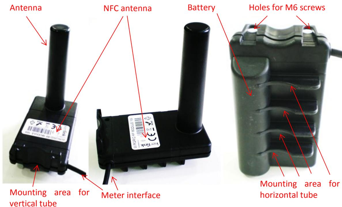
Figure 3: Views of the Wirgrid RF Module 169MHz
