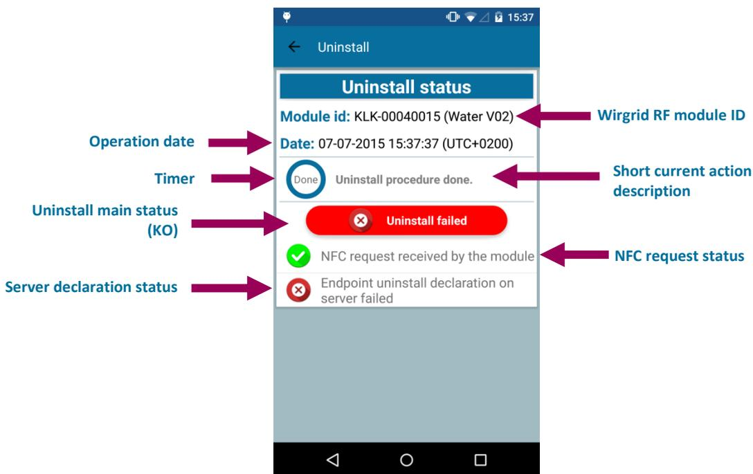
Figure 37: Uninstall failure (Server declaration failure)
