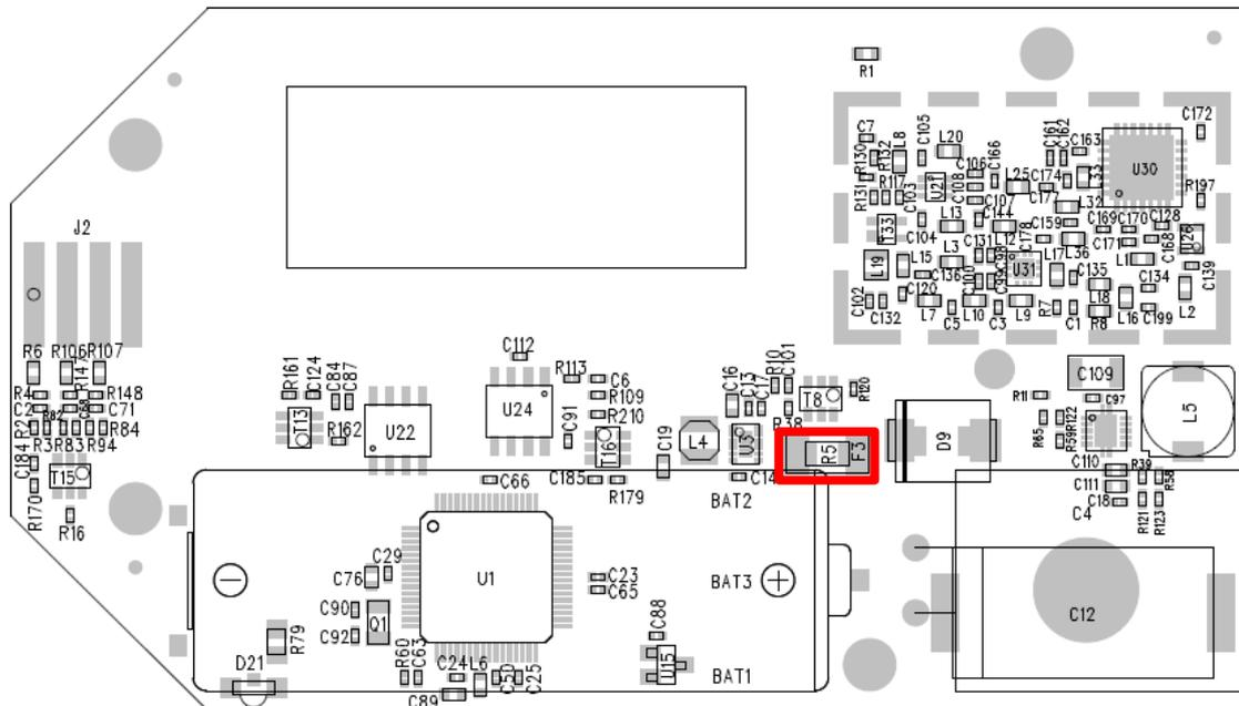
Figure 42: Position of the F3 fuse in the Wirgrid RF Module 169MHz
