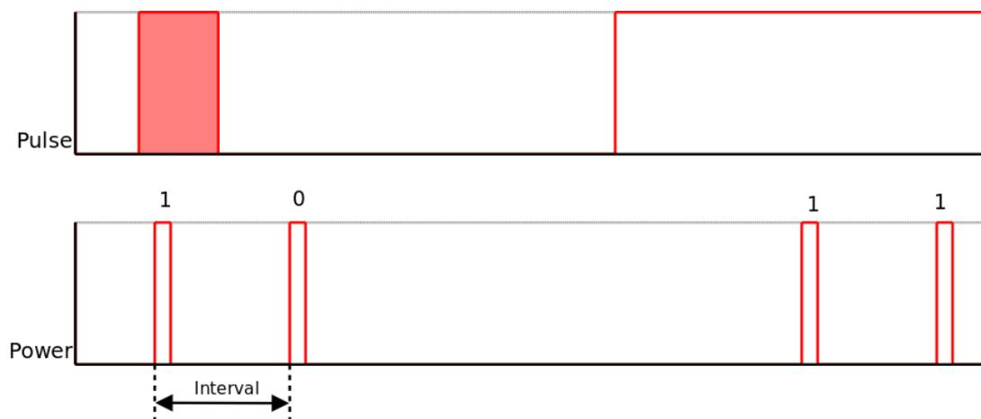
Figure 22: Advanced pulse counter glitch filtering
