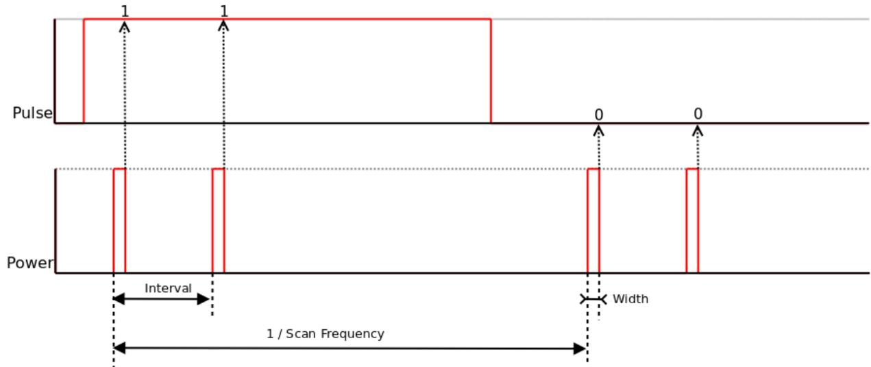
Figure 21: Advanced pulse counter sampling
