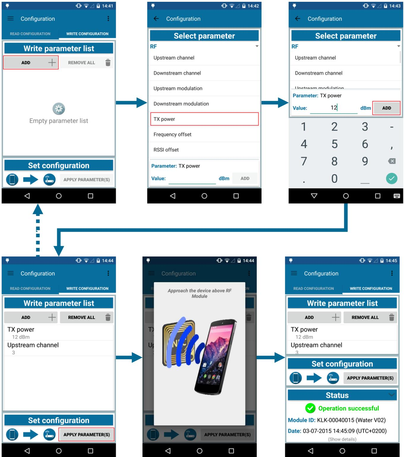
Figure 26: Write configuration operation
