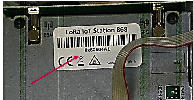
Figure 6: Wirnet Station Board ID
