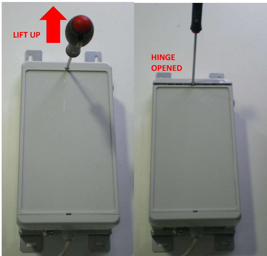
Figure 11 : Opening of the compact enclosure with screwdriver
