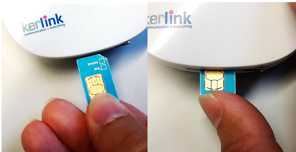
Figure 101: Position of the USIM card before insertion into the USIM connector
