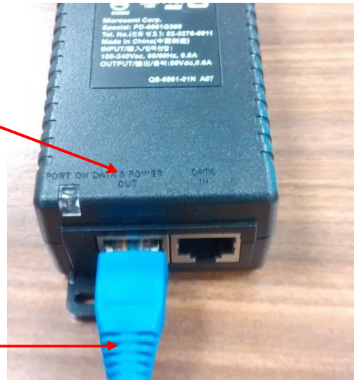
Figure 147 : Ethernet connection on PoE injector side
