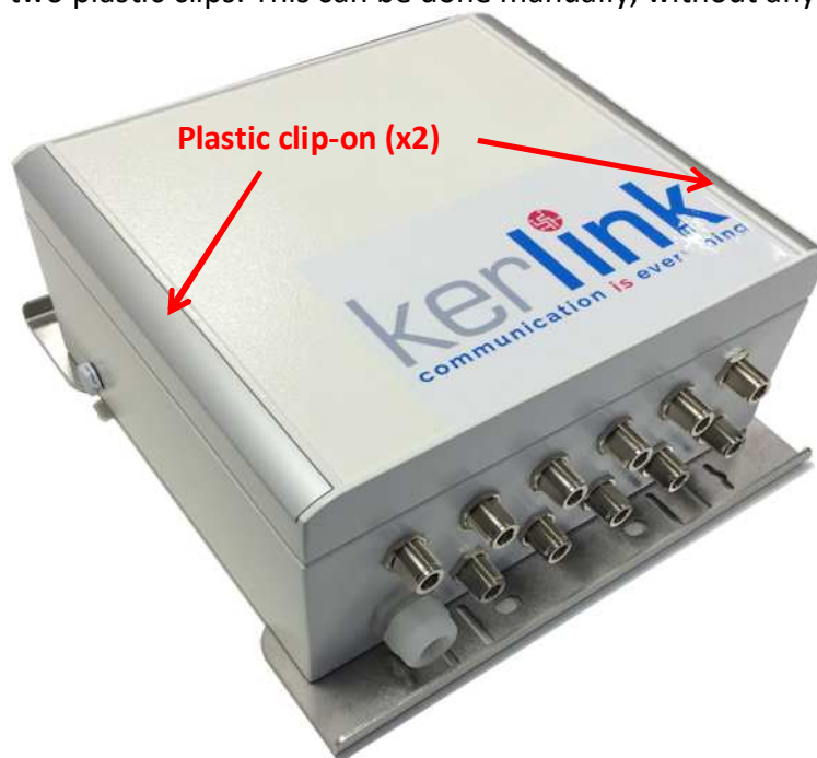
Figure 84: Wirnet iBTS – plastic clips on the lid
