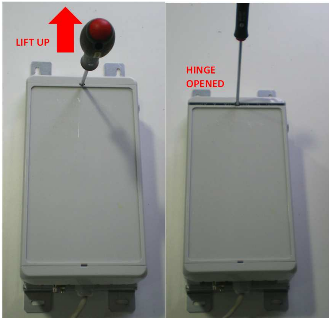
Figure 87 : Opening of the compact enclosure with screwdriver
