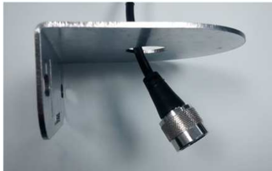
Figure 97 : N connector introduced in the hole of the dome antenna bracket
