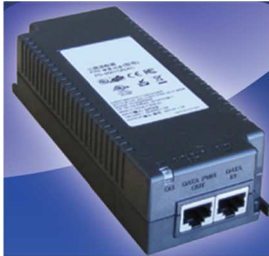
Figure 29 : indoor 60W AC/DC POE injector
