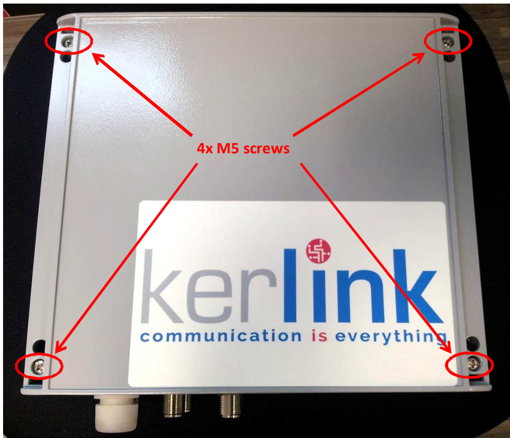
Figure 85: Wirnet iBTS – 4x M5 screws
