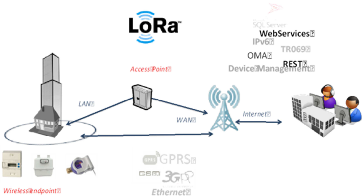
Figure 1: LoRa Network topology
