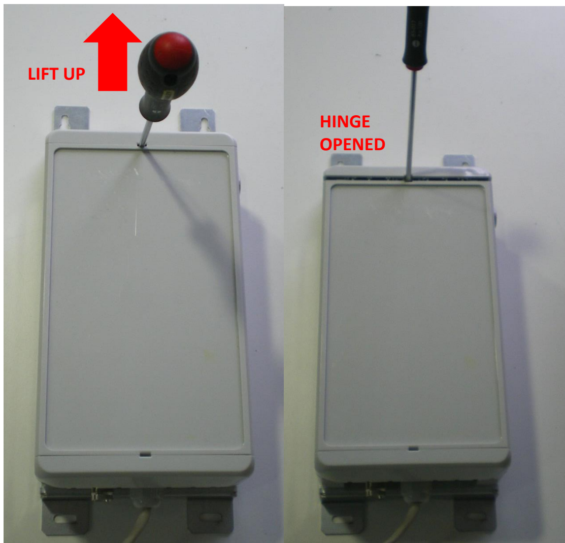
Figure 11 : Opening of the compact enclosure with screwdriver
