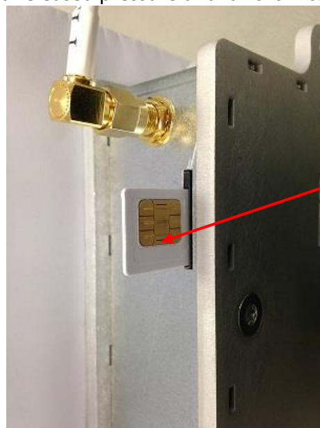
Figure 12 : USIM Card – Wirnet iBTS
