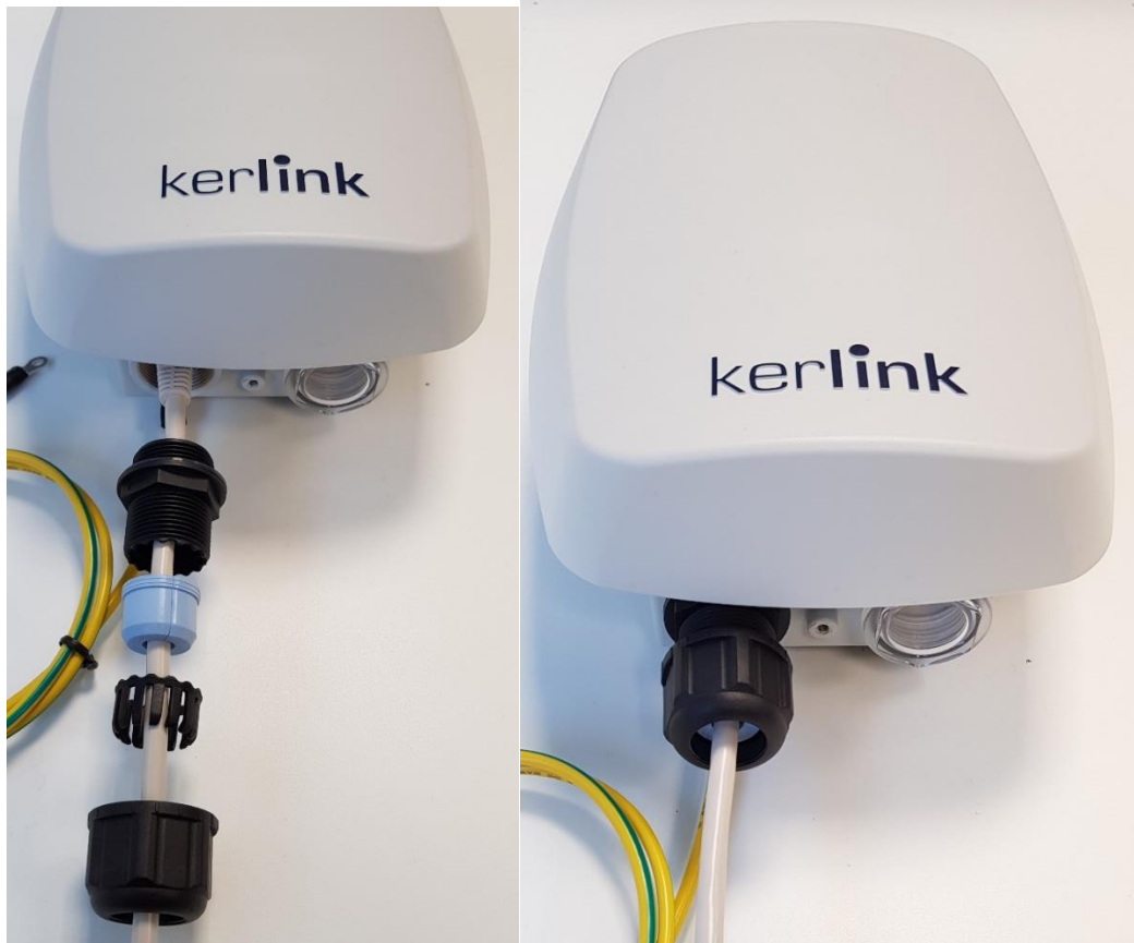
Figure 84 : Wirnet iStation Ethernet connection
