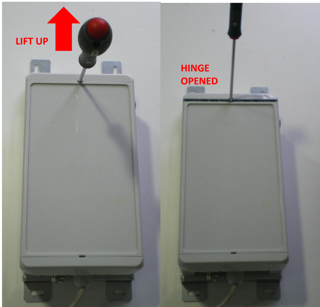
Figure 11 : Opening of the compact enclosure with screwdriver
