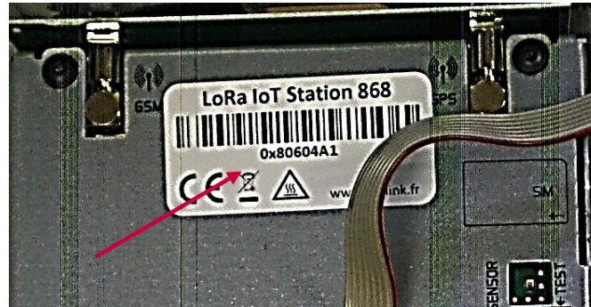
Figure 6: Wirnet Station Board ID
