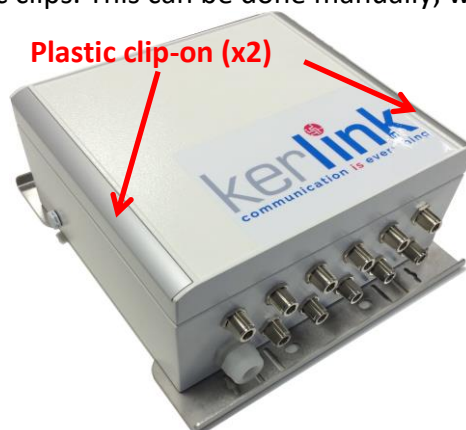
Figure 8: Wirnet iBTS – plastic clips on the lid
