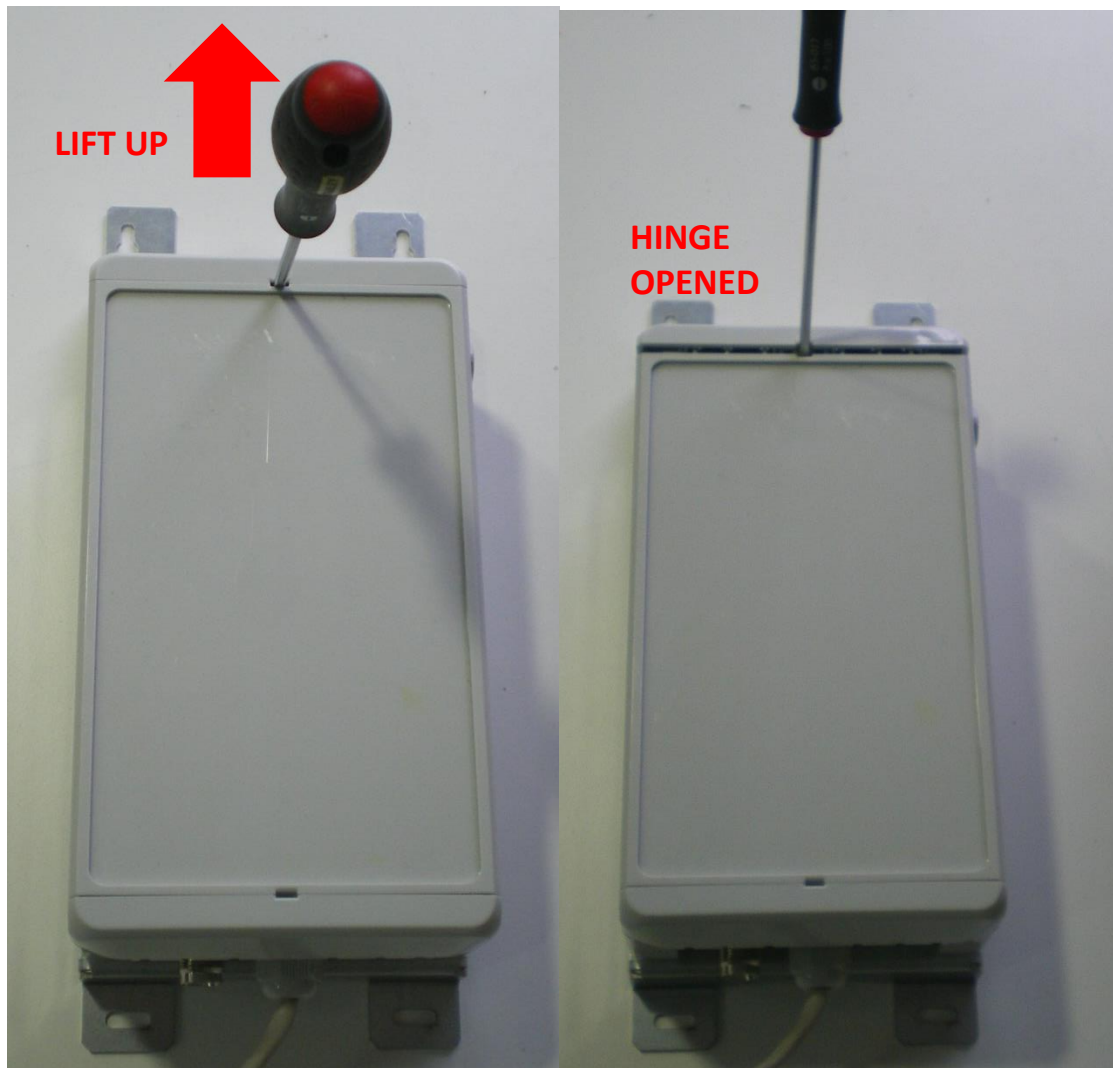
Figure 11 : Opening of the compact enclosure with screwdriver
