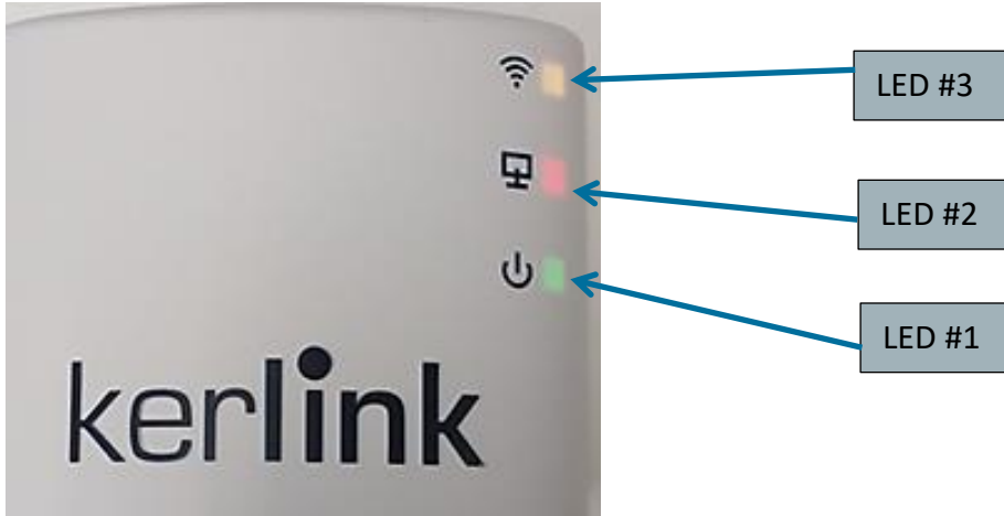
Figure 117: View of LEDs
