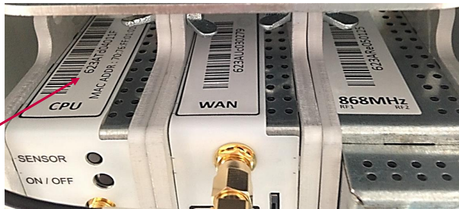
Figure 5: Wirnet iBTS Board ID
