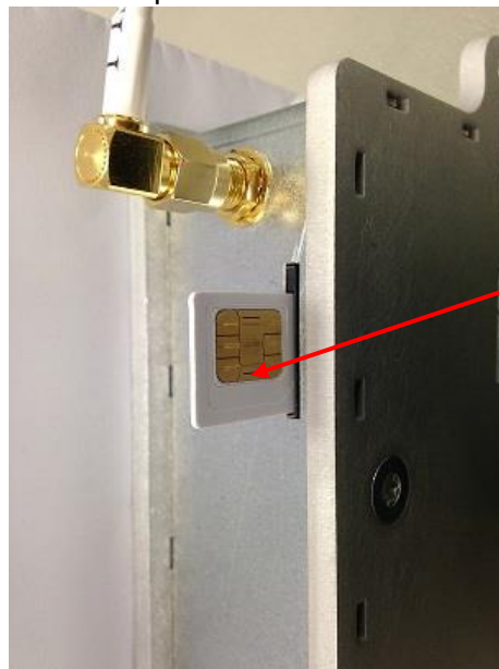
Figure 12 : USIM Card – Wirnet iBTS
