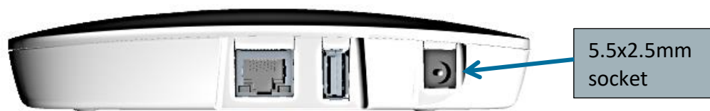
Figure 114: View of the 5.5x2.5mm socket
