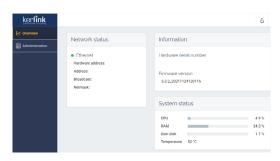
The generic syntax for web interface is http://klk-zeth-<serial>/ Serial is the last digits of the gateway EUI (available on the gateway Identification Card) (ex: if gateway EUI is 7076FFyyzz040001: http://klk-zeth-040001/)
