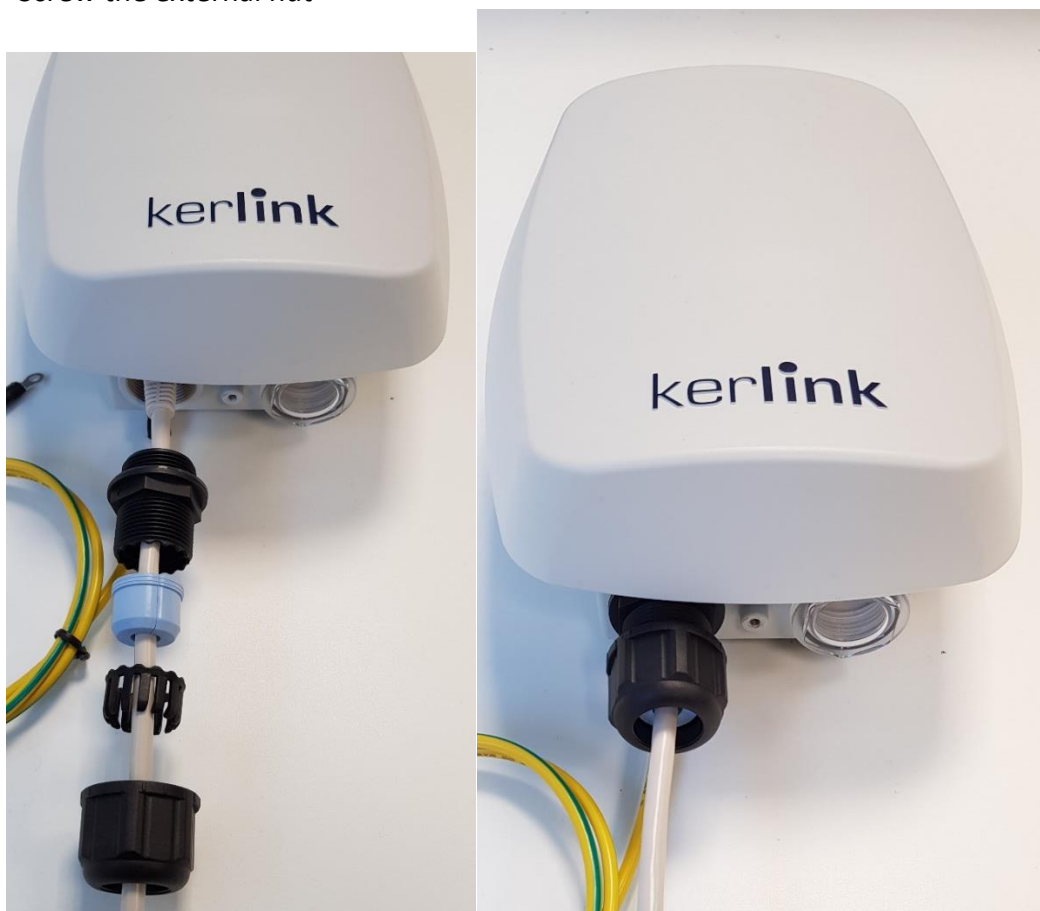
Figure 86 : Wirnet iStation Ethernet connection
