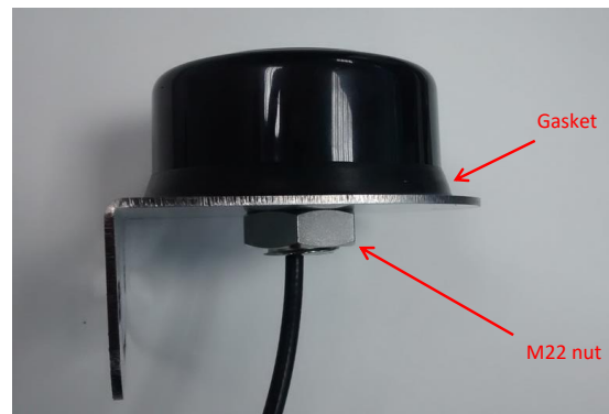
Figure 24 : N connector introduced in the hole of the dome antenna bracket / Figure 25 : Antenna installed on the dome antenna bracket
