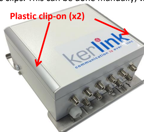
Figure 8: Wirnet iBTS – plastic clips on the lid
