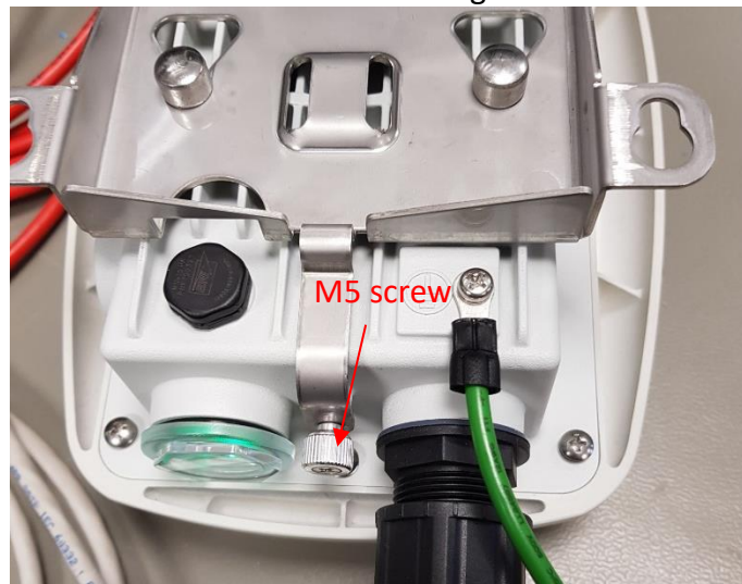
Figure 40 : Detail of M5 screw
