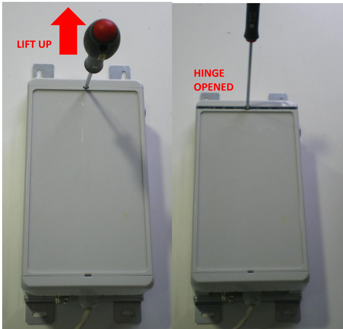
Figure 11 : Opening of the compact enclosure with screwdriver
