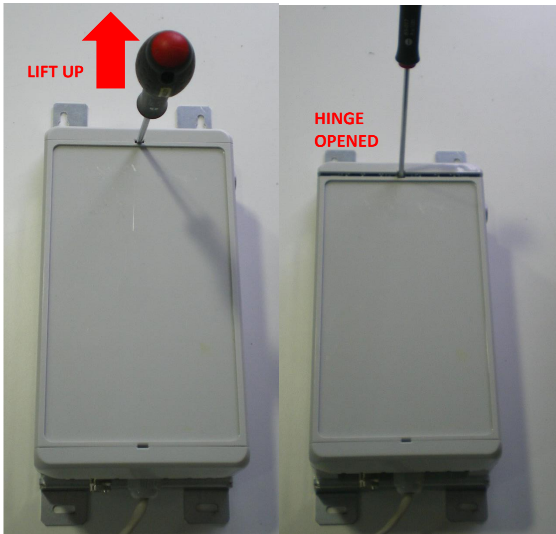
Figure 11 : Opening of the compact enclosure with screwdriver
