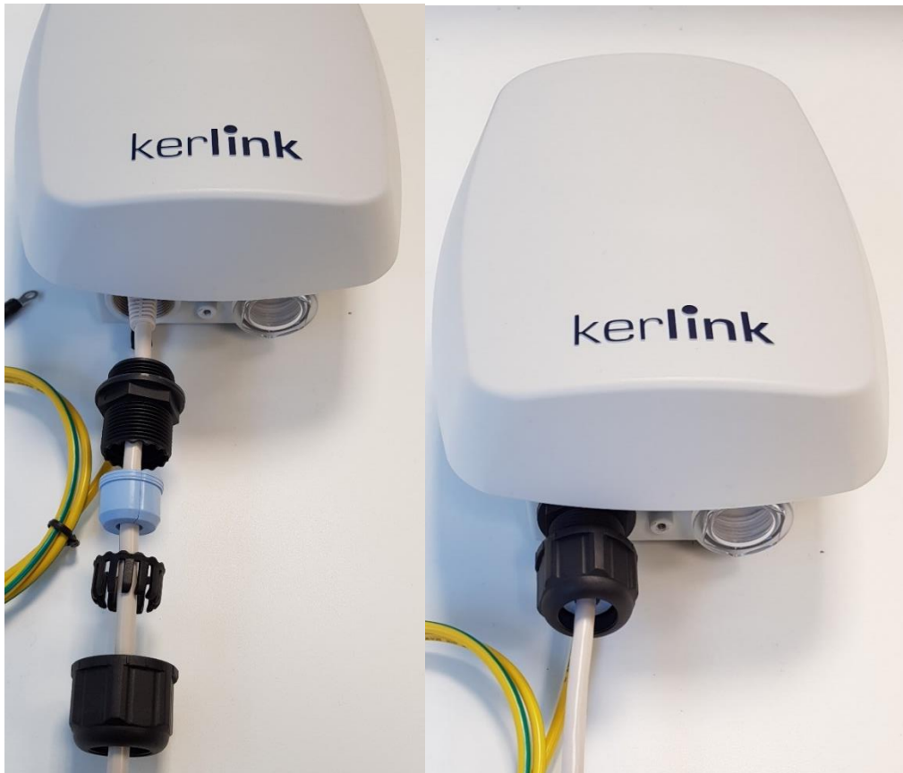
Figure 86 : Wirnet iStation Ethernet connection
