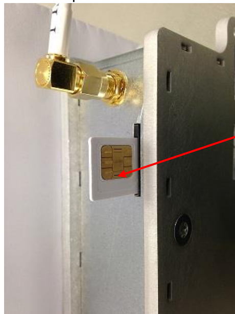
Figure 12 : USIM Card – Wirnet iBTS
