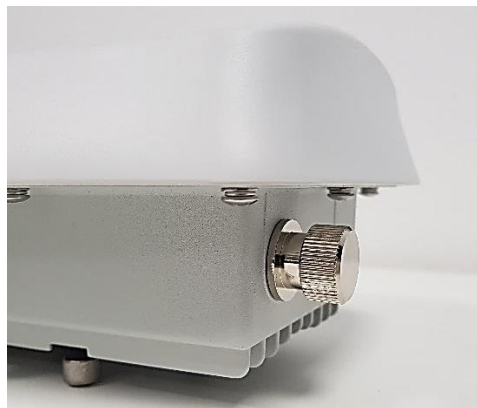
Figure 78 : LoRa antenna port with N cap
