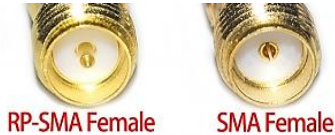
Figure 107: Differences between RP-SMA female and SMA female connectors
