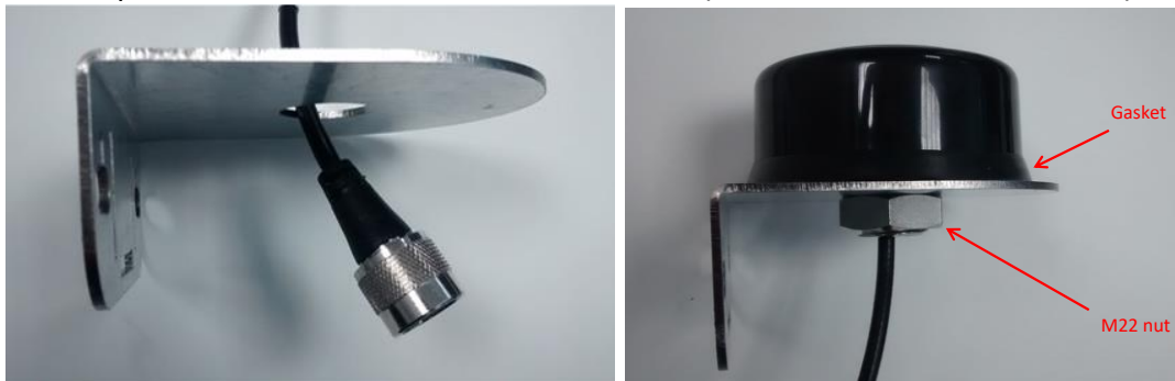
Figure 24 : N connector introduced in the hole of the dome antenna bracket / Figure 25 : Antenna installed on the dome antenna bracket
