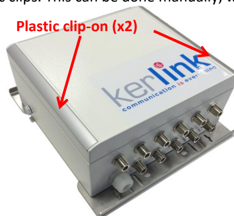
Figure 8: Wirnet iBTS – plastic clips on the lid
