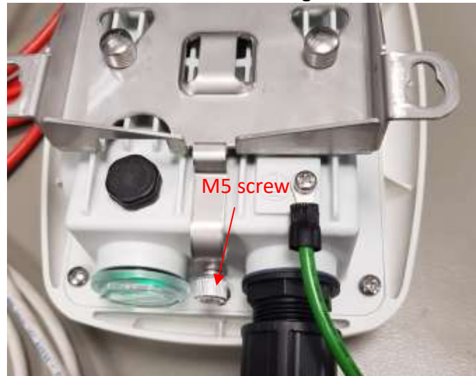
Figure 40 : Detail of M5 screw
