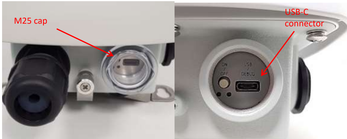
Figure 95: USB interface on bottom side – Wirnet iStation
