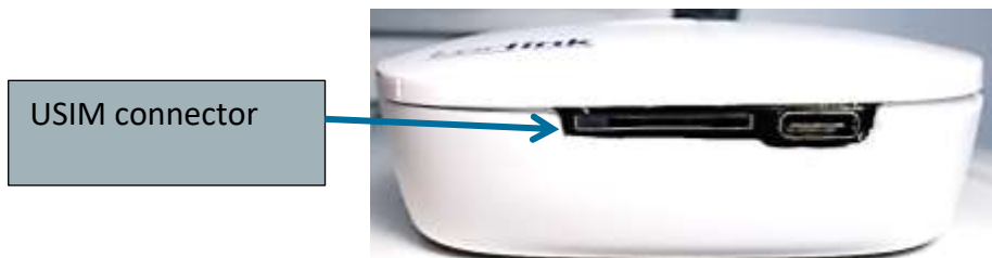
Figure 100: Views of the USIM connector
