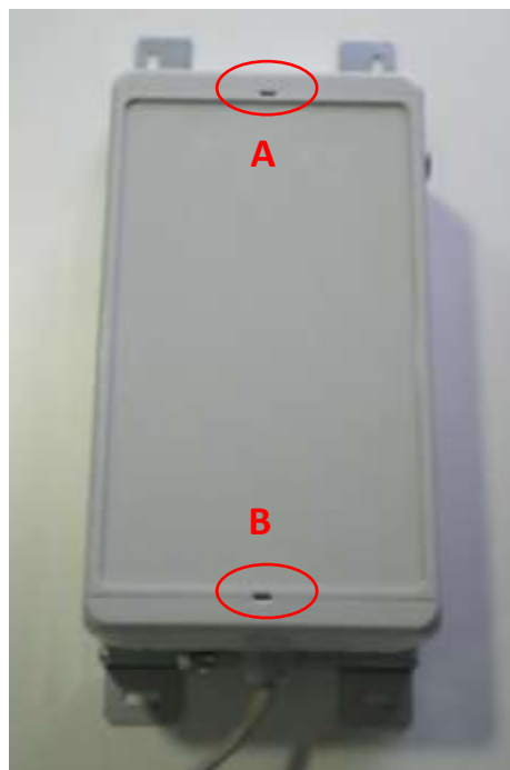
Figure 10 : Open points of the compact enclosure
