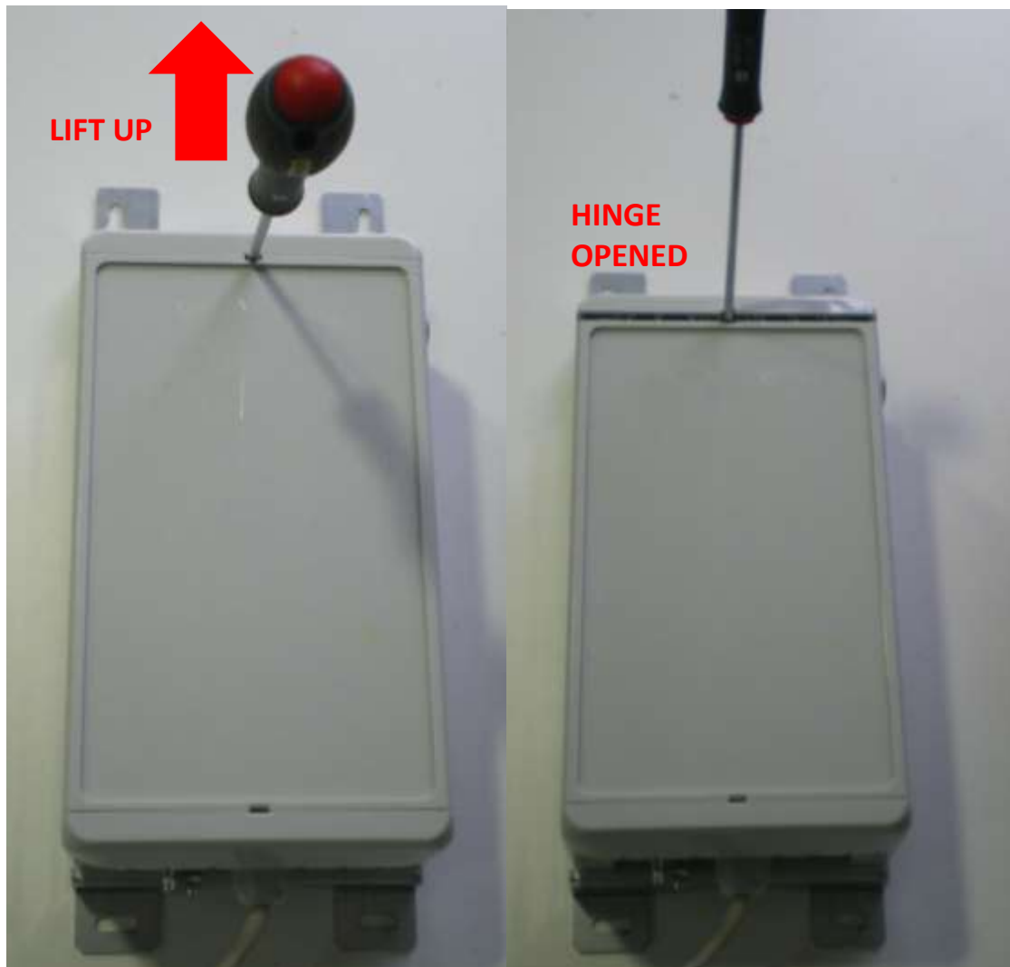
Figure 11 : Opening of the compact enclosure with screwdriver
