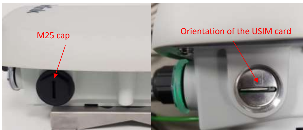
Figure 14 : USIM Card insertion – Wirnet iStation
