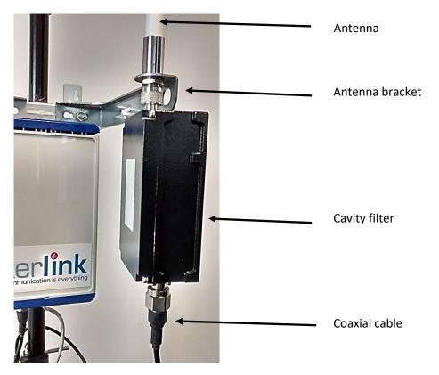
Avoid direct mounting on the gateway since the weight of the cavity filter may deform enclosure.
