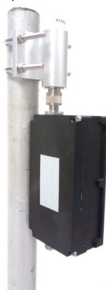
Screw the cavity filter onto the antenna through the N connector
