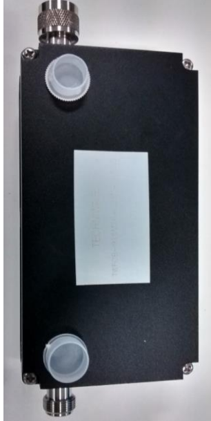
Remove caps on both N connectors
