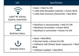
Indicative timings: • SW reset takes around 1min 30s • Boot takes around 1min 20s, • Backhaul connection takes around 10s,
