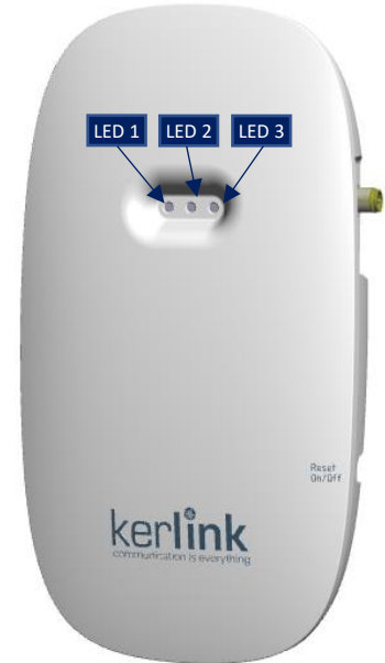
Figure 2: Wirnet iFemtocell LEDs
