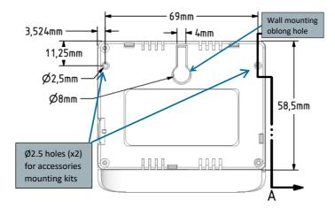
Two non-threated holes (2.5mm diameter, 6mm depth) could be also used for accessories mounting. Plastic screws with 3mm outside thread and 2.1mm core thread are recommended.
