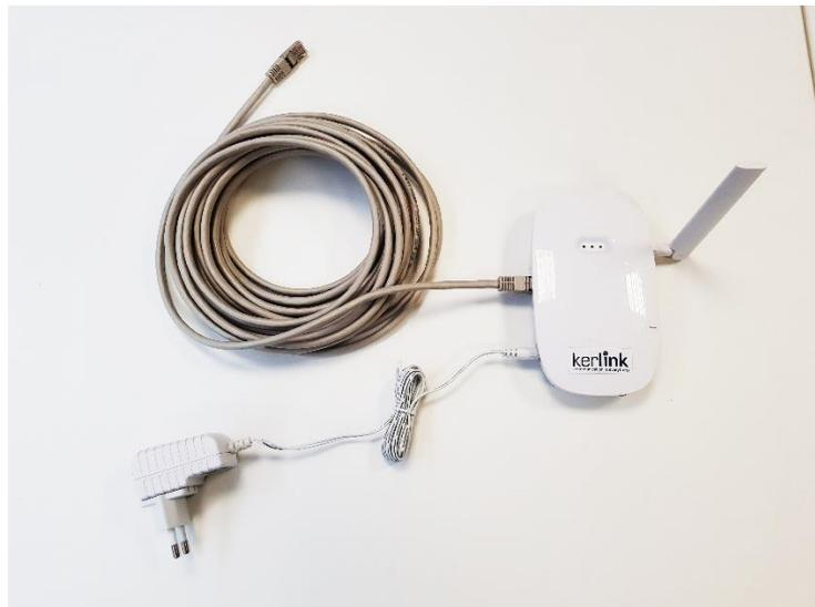
*Figure 1: Wirnet iFemtocell setup (EU version pictured)*
